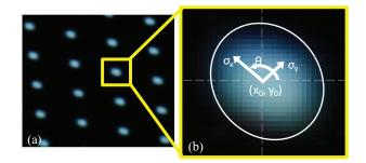
Fig. 6. Projector pixel modeling. (a) Projector pixels from an acquisition pattern image used to estimate metapixel parameters. (b) Close-up of a projector pixel on the camera plane and the five metapixel parameters to be discovered.
